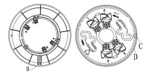
The flashing beacon base does not require cabling. It will share the termination of the detector.
